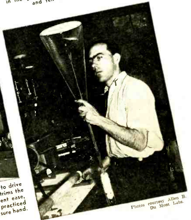
Examining the C-R tube with a polariscope to detect strains in the glass. Various hues indicate stress or strain in the glass and tell whether a tube should be rejected.
