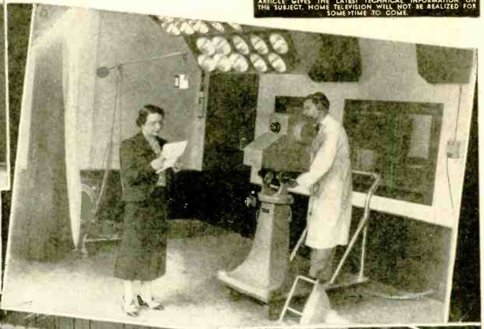
Right—A view in one of the television studios where an iconoscope picks up the image. Note the mike suspended above the speaker.
