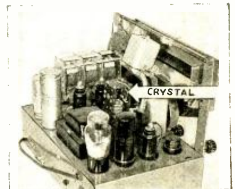
Fig. 7, below—Chassis of standard American 7-tube superhet. fitted with wedge-crystal. Wedge-shaped crystals when available can be installed at slight cost, with great-boost in tone quality and selectivity.
